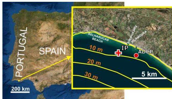
Figure 1. Location of the tracer injection point (IP) and the Acoustic Doppler Current Profiler position (ADCP). Depth contour lines on the right map are referred to hydrographic zero.
